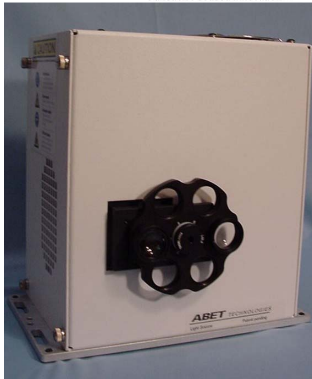
LS-150-Xe light source with FW-LS filter wheel with two condenser lenses loaded
